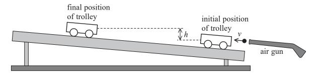
The pellet was fired into the trolley, and h measured, several times. A mean value of h was calculated.
