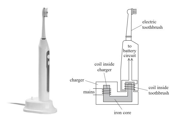
The charger contains a coil wrapped around an iron core. The coil is plugged into the mains supply. The toothbrush also contains a coil that sits around the iron core when the toothbrush is placed on the charger.
